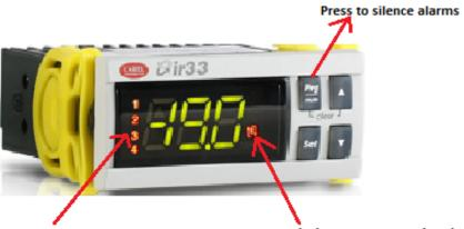
These icons indicate the controller is calling for an output activation. The number lighted corresponds to the numbered output on the
